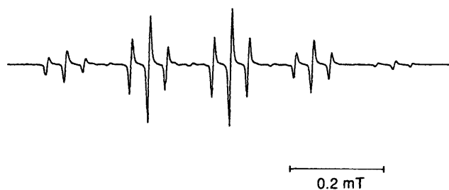
Fig. 2 EPR spectrum of 1 •- in CH 2 Cl 2 at -80 °C. The g value is 2.003 43. On the high-field side the spectrum is a little weakened in intensity, probably because of the decay of the radical.
